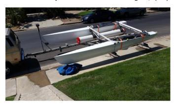
carried to the main beam attachment molding and to the truss as it splits around the centerboard trunk. I did it this way to make the hull forward of the main beam VERY stiff. i can detect no flex of the hulls on high wind sailing. There is no foam flotation in the bow since the hulls are wood and will float on their own if holed. The deck is 3/16 okoume plywood sitting on ribs
